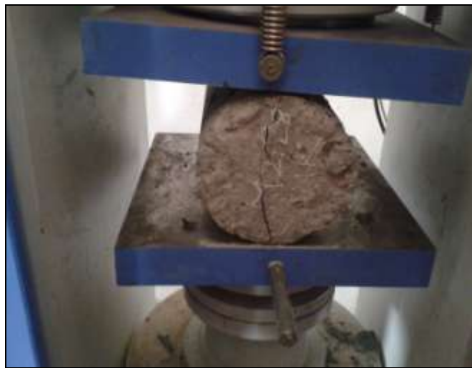
Fig 1.5 split tensile testing of specimen
