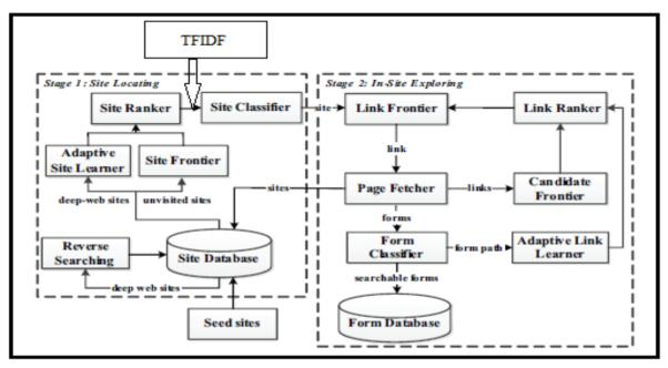
Figure 1. Architecture Diagram
