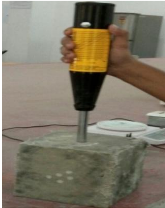
Fig 8: Rebound hammer test on cube specimen
