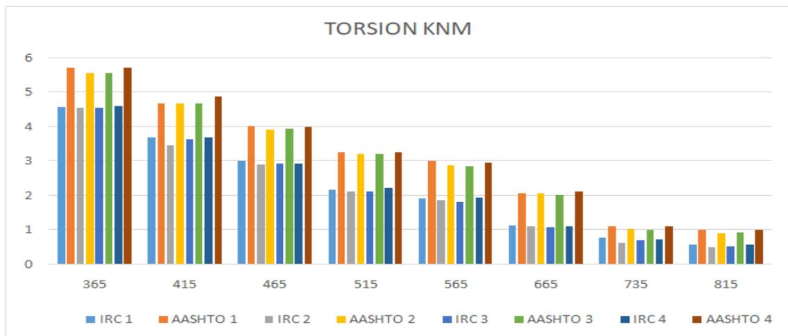
FIGURE 4 : VARIATION OF TORSION IN CONCRETE GIRDERS
