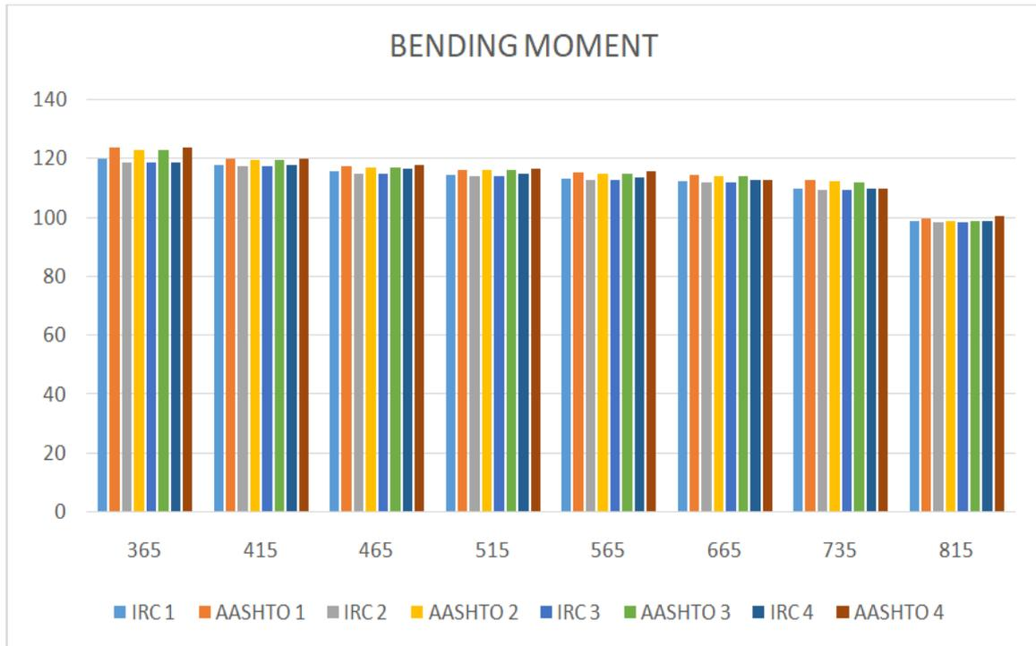
FIGURE 5 : VARIATION OF BENDING MOMENTS IN CONCRETE GIRDERS
