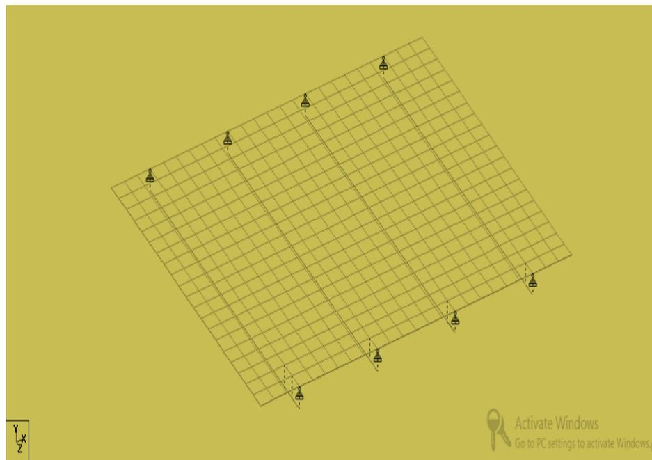
FIGURE 3: Isometric View of concrete slab and four supporting girders (480 plates)
