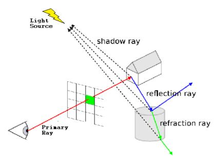
Figure 1.Image of sphere is createdon image plane by ray tracing rays [3]
