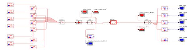
Fig 1. Experimental set up for 96 channel WDM system with RZ modulation format
