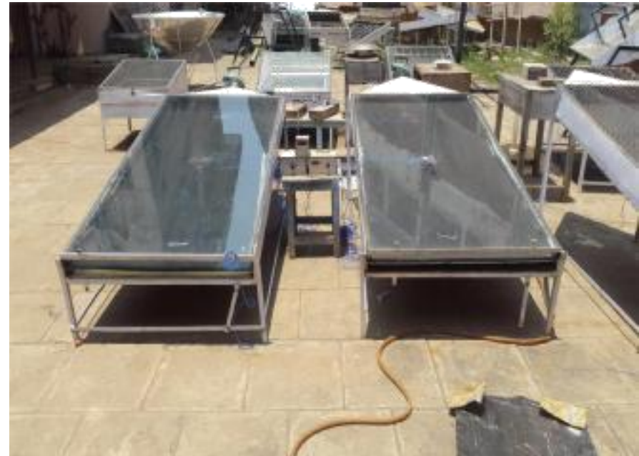
Fig 3.3 Photographic view of experimental set up two different air heaters
