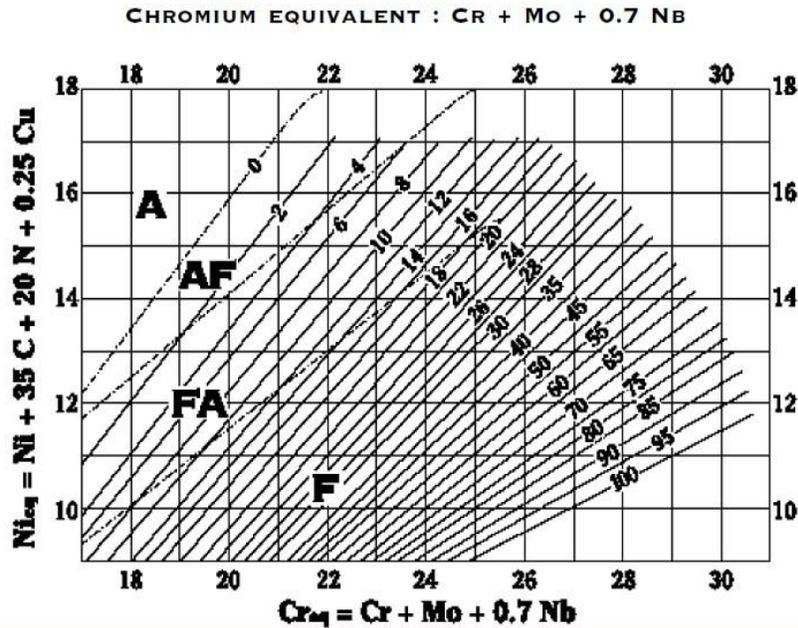
Fig. 2(b) WRC-1992 DIAGRAM source [25]
