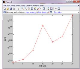
Fig 10: BER performance of Log distance shadowing propagation model
