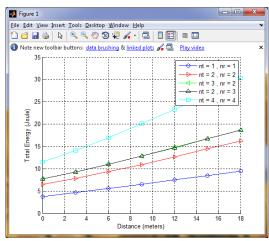
Fig 2: Graph between energy of signal and distance of Friis propagation model
