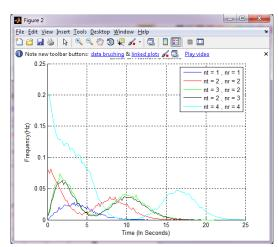
Fig 3: Graph between spectrum frequency and time of Friis propagation model.
