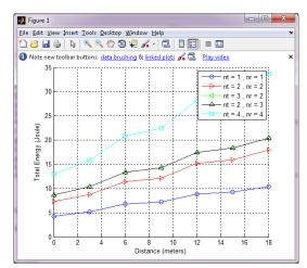
Fig 6: Graph between energy of signal and distance of Log distance shadowing propagation model
