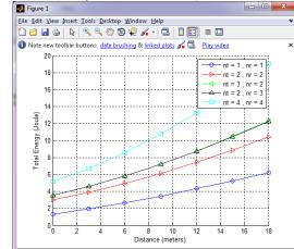
Fig 4: Graph between energy of signal and distance of Rayleigh propagation model
