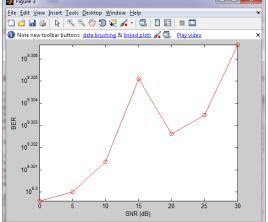
Fig 9: BER performance of Rayleigh propagation model
