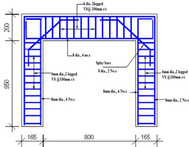
**Fig.4: Inverted L- type detailing arrangement with splay steel (SP3)**
