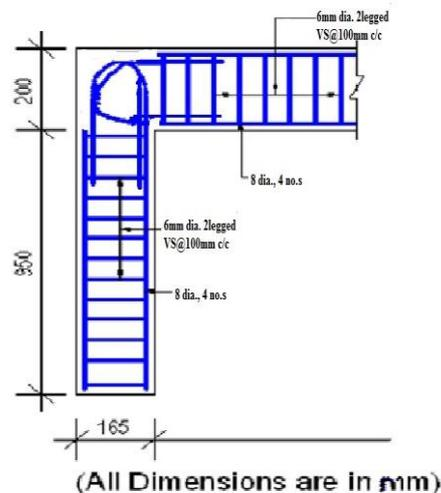
**Fig.5: Overlapping U Stirrups type detailing arrangement (SP4)**
