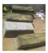
Specimen type B1, B2, B3 and B4 is control beam, one layer at bottom, two layer and three layer at bottom of CFRP sheet. And after 28 days flexural strength measure.
