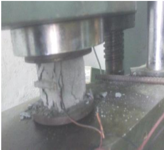
Figure. 2 Testing For Compressive Strength
