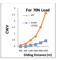
Fig. 5 cu mu lative wear volume for the uncoated, the detonation sprayed  $Al_2O_3$ -13Ti $O_2$  coated MS steel subjected to wear at normal loads of 50N, 60N and 70 N and sliding velocity of 1m/sec.
