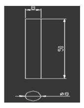
Fig. 2 Sketch of pin (specimen) used for pin-on-disc wear test
