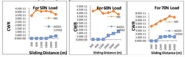
Fig. 4 cumulative wear rate for the uncoated, the detonation sprayed Al<sub>2</sub>O<sub>3</sub>-13TiO<sub>2</sub> coated MS steel subjected to wear at normal loads of 50N, 60N and 70 N and sliding velocity of 1m/sec
