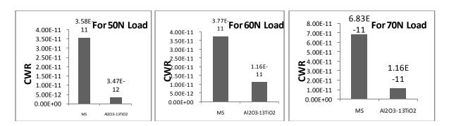
Fig. 5 Cumulative wear rate for the uncoated, the detonation sprayed Al<sub>2</sub>O<sub>3</sub>-13TiO<sub>2</sub> coated MS steel subjected to wear at normal load of 70 N and sliding velocity of 1 m/sec after a sliding distance of 5400 meters.
