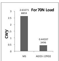
Fig. 7 Cumulative wear rate for the uncoated, the detonation sprayed Al<sub>2</sub>O<sub>3</sub>-13TiO<sub>2</sub> coated MS steel subjected to wear at normal load of 50N, 60N and 70 N and sliding velocity of 1 m/sec after a sliding distance of 5400 meters.
