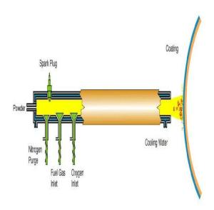
Fig.1 Schematic diagram of the D-gun spray process.
