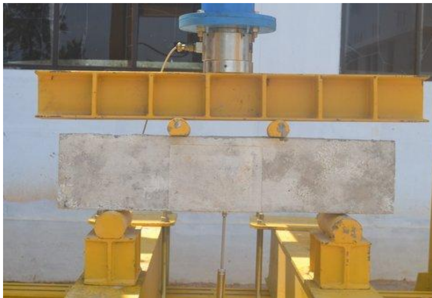
Figure-12 Load deflection test set up
