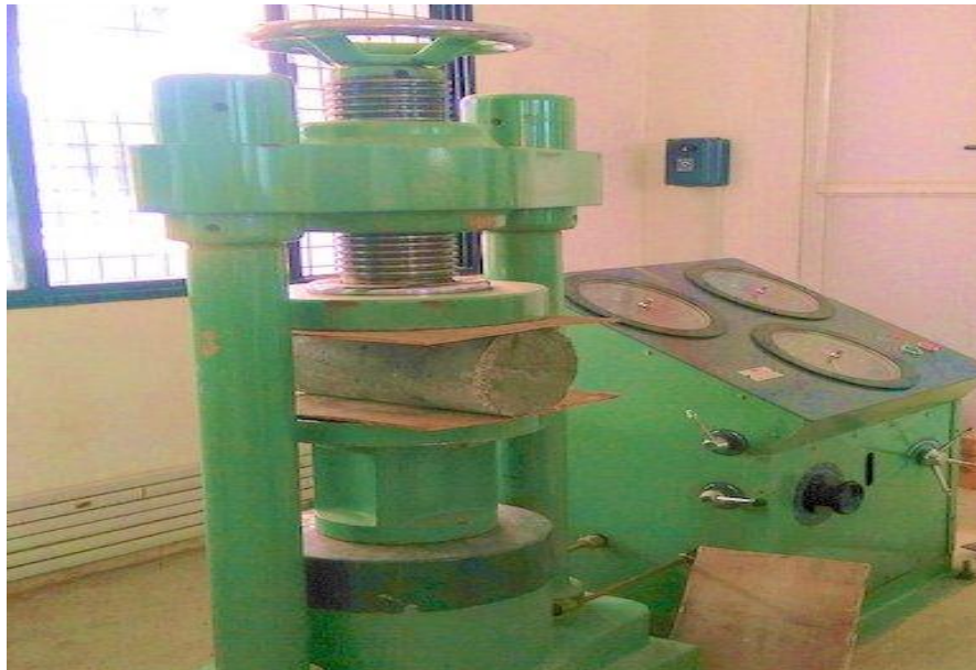
Figure-7 Split tensile strength on cylinder
