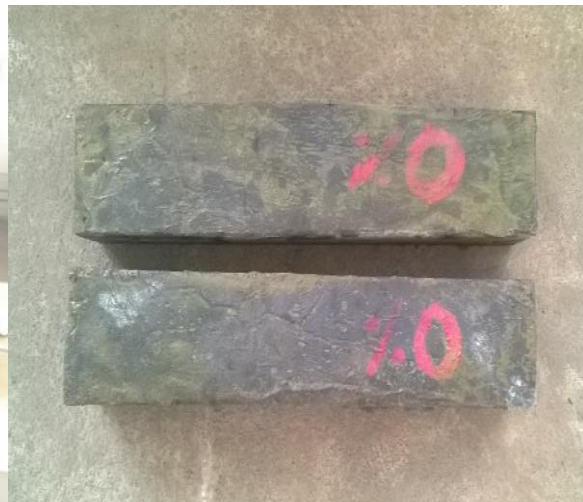
Figure-5 Test Beam specimen
