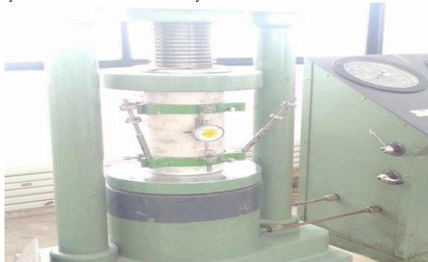
Figure-8 Experimental set up for finding modulus of elasticity
