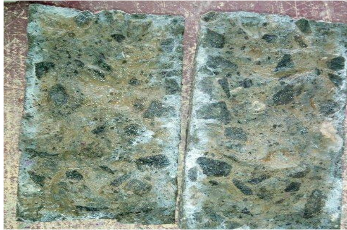
Figure-11 Specimen for bulk diffusion test
