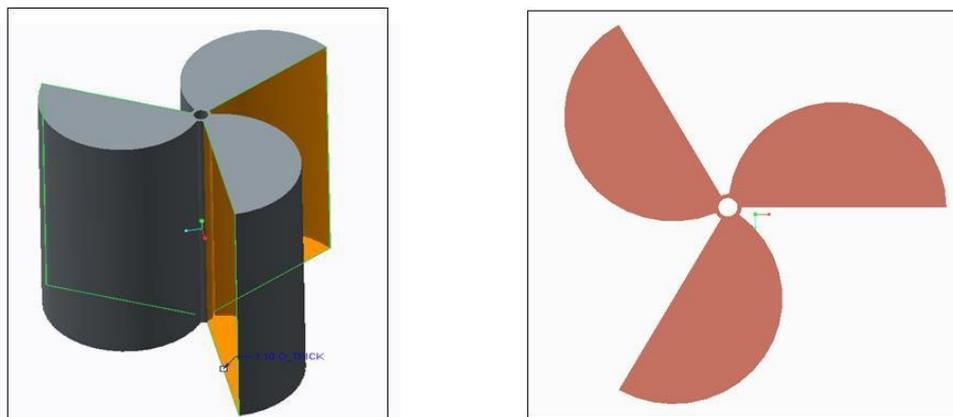
**Figure 7. Savonius Wind Turbine Model with Rotor**
