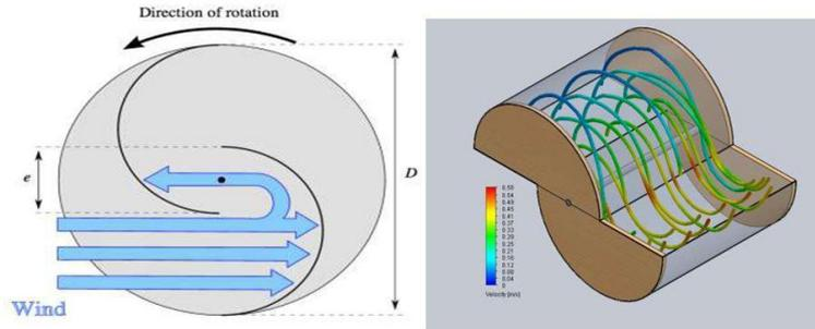
**Figure 2. Wind Rotation in Savonius Turbine**
