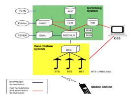
Figure 2. GSM Network Elements
