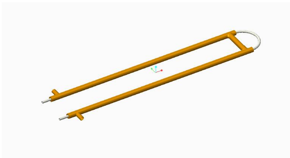
Fig.4.3.2 Model of double pipe heat exchanger
