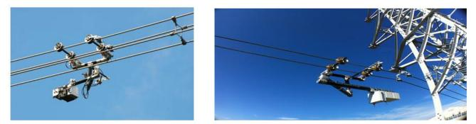
The inspection robot is keep on moving across transmission line back and forth. And at same time monitors the parameters, continue sends the signals to the receiver end. It has two sections: Transmission Sector and Receiver section. Working is explained with the help of basic block diagram as follows:
