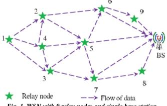
Fig. 1. WSN with 9 relay nodes and single base station.
