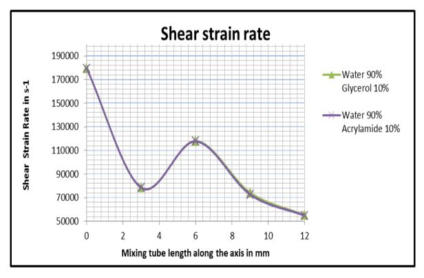
Fig 4.3(a) Shear Strain Rate vs. Mixing Chamber
