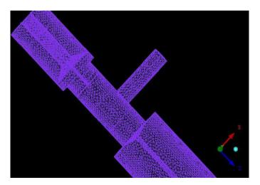
Fig 2 Nozzle Head Model with Mesh
