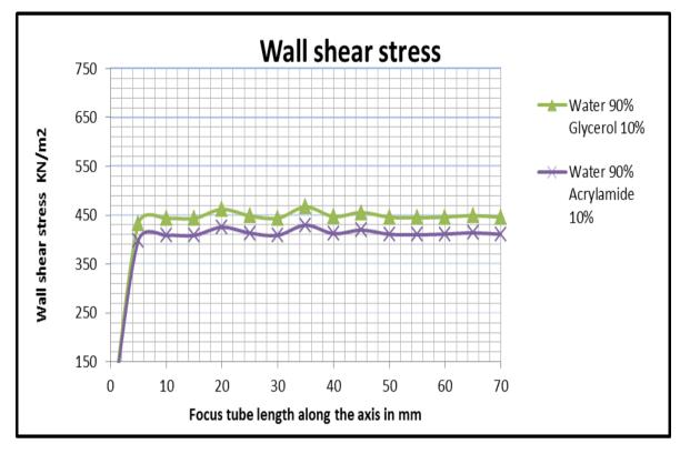
Fig 4.2[b] Wall shear stress vs. Focus tube
