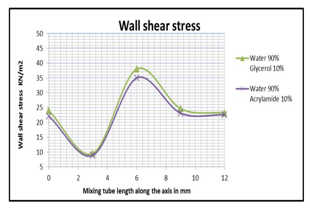
Fig 4.2[a] Wall shear stress vs. Mixing Chamber
