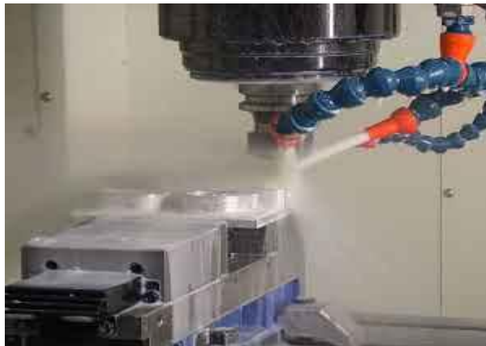
Figure no:-2.1 – coolant being used in machining (CNC)
