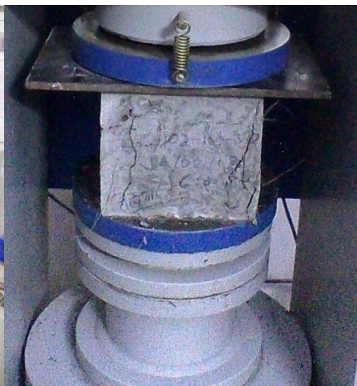
fig-2, crushed cube specimen
