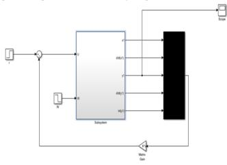
Figure: (ii) MATLAB model of Active Suspension System
