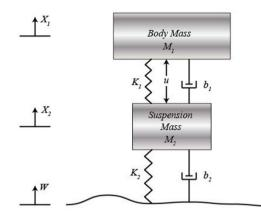
Figure: (i) Passive Suspension System
