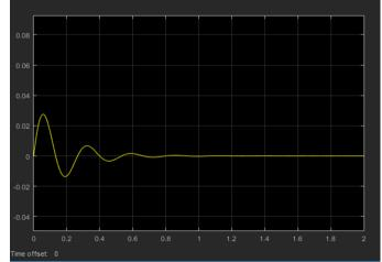
Graph: (iii) Car body displacement for 10 cm step input for active system
