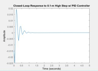
Graph: (ii) Close loop response to 10 cm high step w/ PID controller
