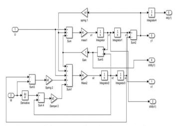
Figure: (iii) Subsystem of Active Suspension System
