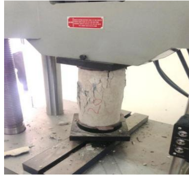
Figure-2: Concrete specimen cylinder under compression testing
