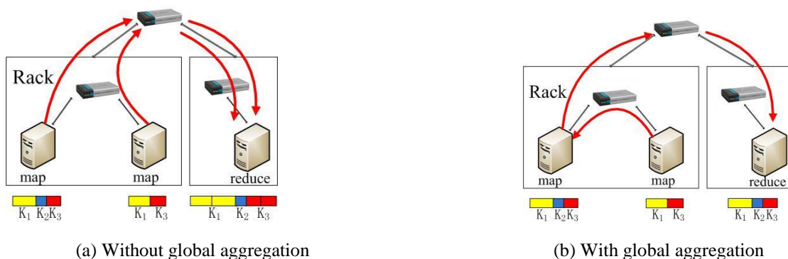
Fig. 2. Two schemes of intermediate data transmission in the shuffle phase.
