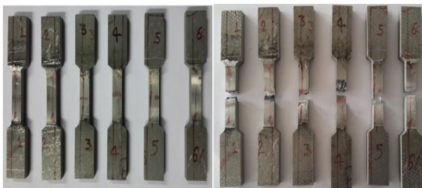
Figure. 8 Tensile specimens (a) before test and (b) after the test
