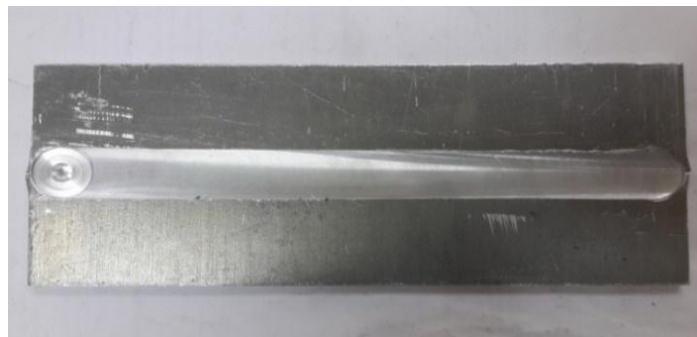
Figure. 5 Friction stir welded Al6082/TiC plate
