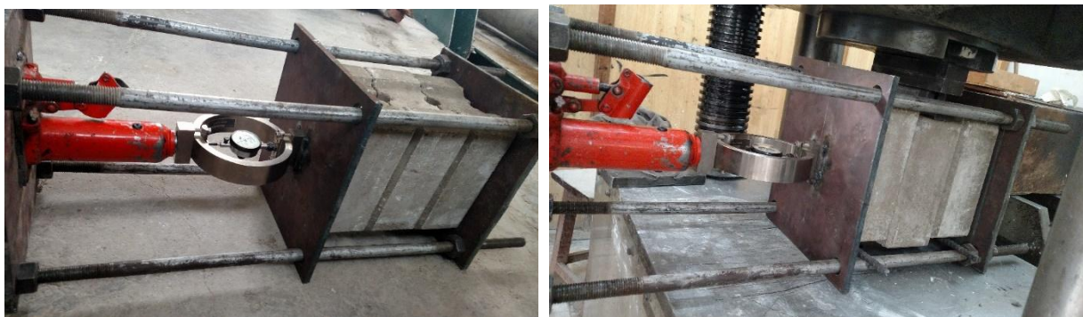
Figure 2 General setup of Triplet Apparatus (left), Middle block sheared in UTM (right)
