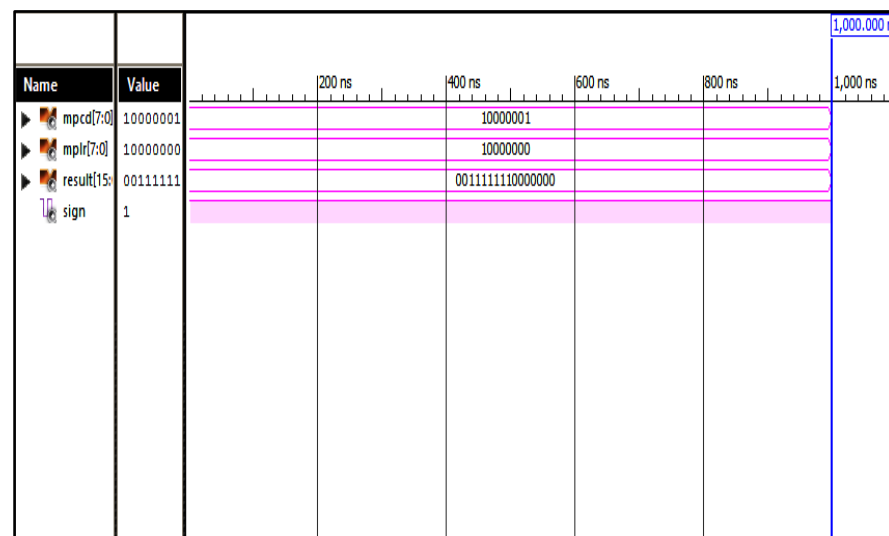
Fig.3.Simulation Result of 8 Bit Multiplier
