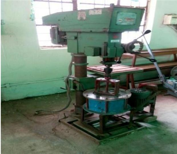
Fig. 3.1 Assembled diagram of slurry pot tester
