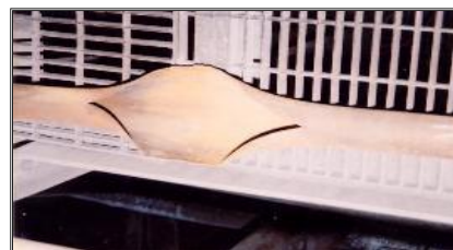
Fig:4 Tube failures because of LTOH.
