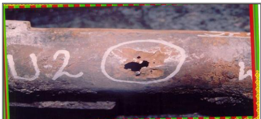
Fig:5 Tube failures due to caustic corrosion.
