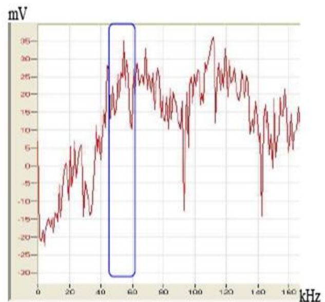
Fig 14 : Spectrum for Leak at pressure chamber
