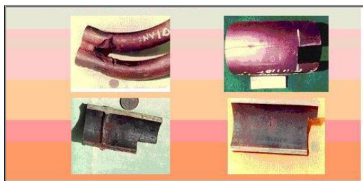
Fig: 7 Tube failures because of fatigue failure
