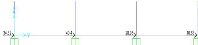
**Figure 4: Application of blast load laterally to the nodes**
