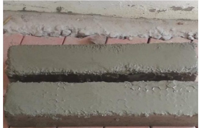
Fig 2: Beam strengthened with steel mesh
