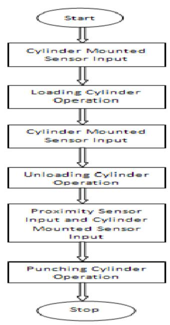
There are three main components used in this system. They are Loading Cylinder, Unloading Cylinder, and the Punching Cylinder. All these cylinders are operated in a sequence in order to perform the required operation
