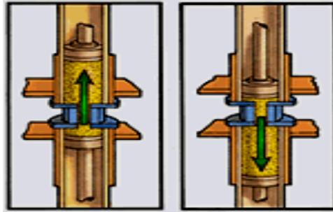
Figure 2 Two-way flow process
