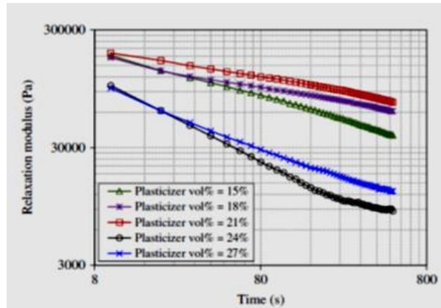
Figure 3 Variation of relaxation modulus with time (Logarithmic scale on both X and Y axes)
