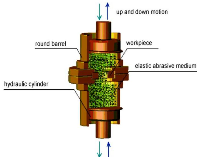
Fig. 5 The machining diagram of AFM
