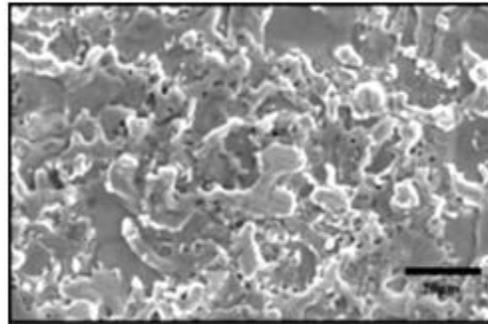
(a) Wire EDM Ra= 2.4  $\mu\text{m}$
