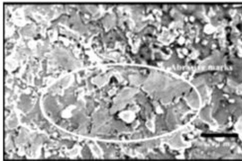
(b) AFMed (150  $\mu\text{m}$ ) Ra=0.8  $\mu\text{m}$
