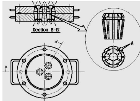
Fig. 6 Deburring process of spring collet
