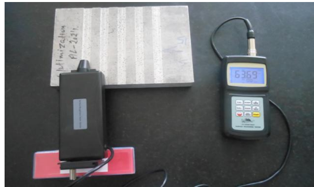
Figure 3 ITI Surftest to measure Surface roughness
