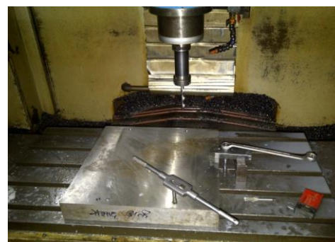
Figure 2 End Milling Operation on Al2024-SiC composite cast plate
