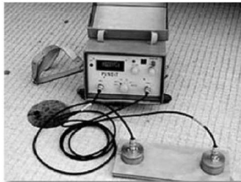
Figure 2 Ultra Sonic Pulse Velocity Test apparatus
