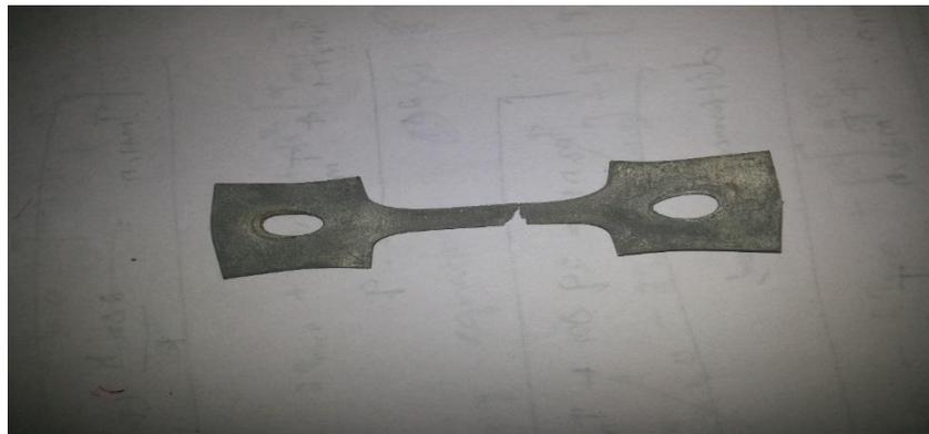
Figure 12. AA5052 (Uniaxial hot tensile test at 560°C)
