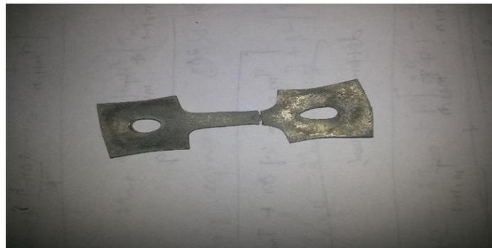
**Figure 4. AA5052 (Uniaxial hot tensile test at 580°C)**
