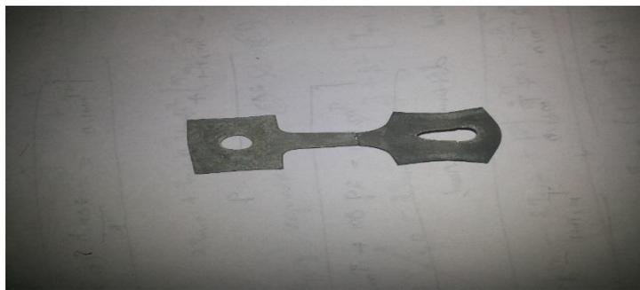
Figure 8. AA5052 (Uniaxial hot tensile test at 570°C)
