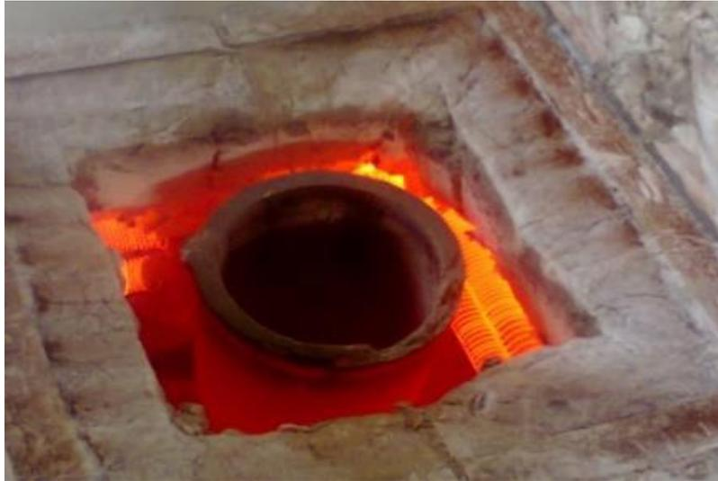
Figure 2. Crucible inside the furnace
