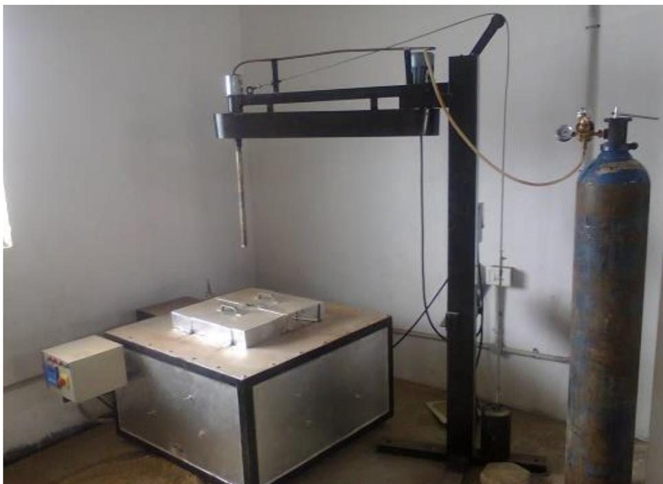
Figure 1. Stir casting equipment
