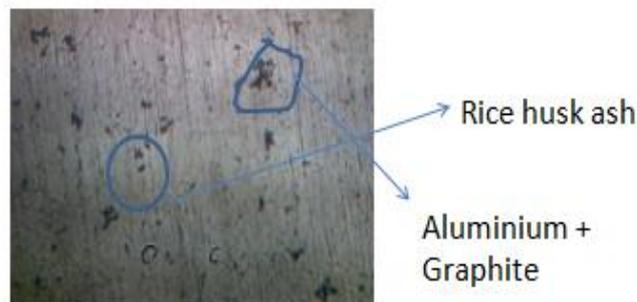
Figure 6. Microscopic observation of 93%Aluminium+5%Graphite+2%Rice husk ash
