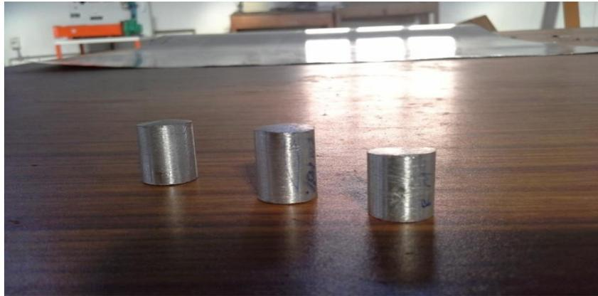
Figure 3. Samples of aluminium, 5% graphite, 2%, 4% and 6% rice husk ash metal matrix composites
