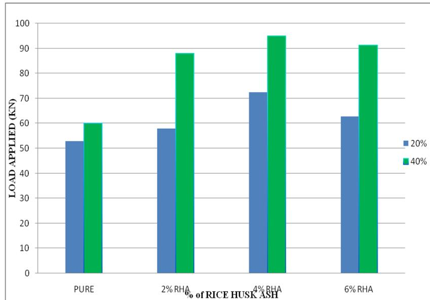
Figure 5. Plot between Load Applied and % Weight Fraction of rice husk ash with aluminium and graphite
