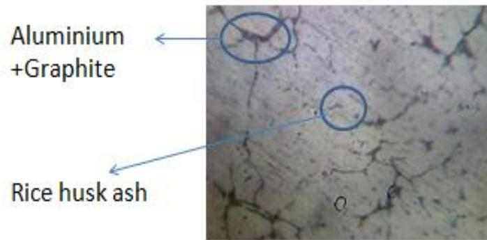
**Figure 8. Microscopic observation of 89%Aluminium+5%Graphite+6%Rice husk ash**
