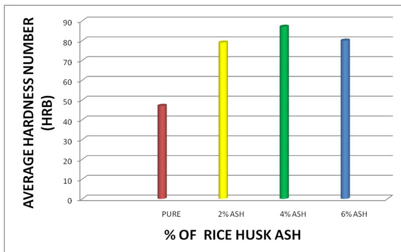
Figure 4. Plot between Average hardness number and % weight fraction of rice husk ash with pure aluminium and 5% graphite.
