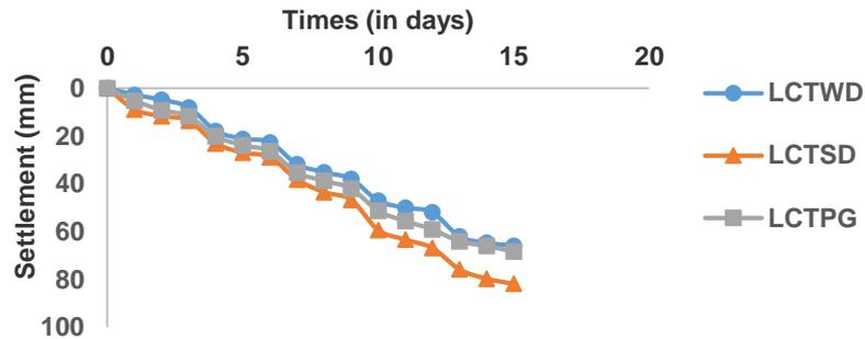
**Fig 6: Settlement versus Time Period In large sized Model Consolidation Test**
