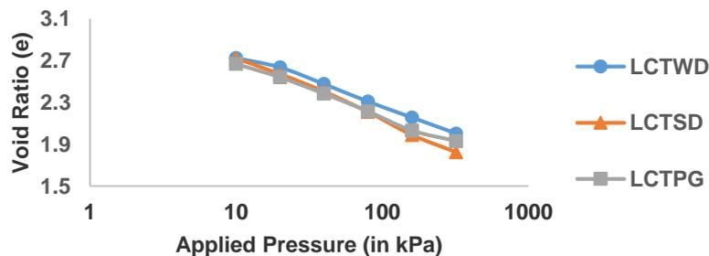
**Fig 8: Comparison of drain material w.r.t. Void ratio (e) against Applied pressure for n=10**
