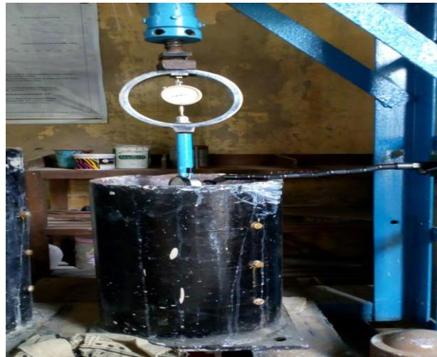
**Fig 1: Large scale Consolidation Test Setup**
