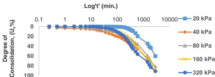
Fig 2: Degree of Consolidation ( $U_v$ ) vs.  $\text{Log}'t'$  for LCTWD
