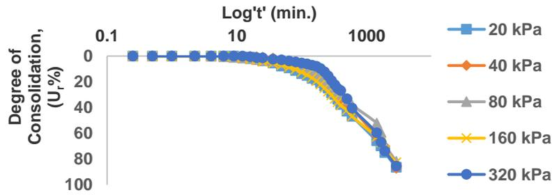
Fig 3: Degree of Consolidation ( $U_r$ ) vs. Log't' for LCTSD
