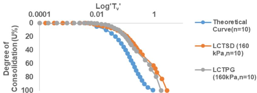
Fig 5: Degree of consolidation versus Logarithmic time factor (for  $n=10$ )
