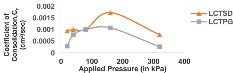
**Fig 7: Coefficient of consolidation through radial drainage ( $C_r$ ) versus Applied Pressure**
