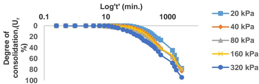
Fig 4: Degree of Consolidation ( $U_r$ ) vs. Log't' for LCTPG
