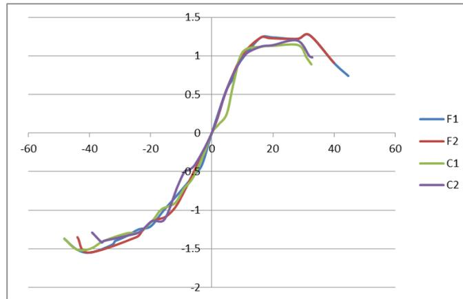
Figure 6. Comparison of peak lateral loads-lateral displacement of the specimens
