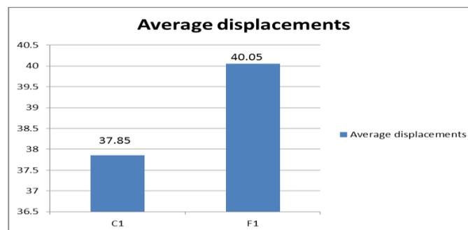
**Figure 5. Comparison on maximum lateral displacement among the specimens**
