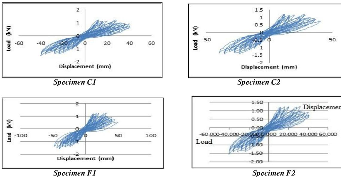
Figure 3. Load displacement curves for the test specimens (for specimens C1,C2,F1&F2 respectively)
