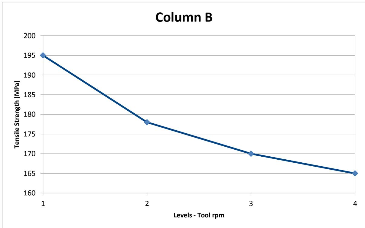
Fig. 1(b): Tensile strength as a function of tool rpm
