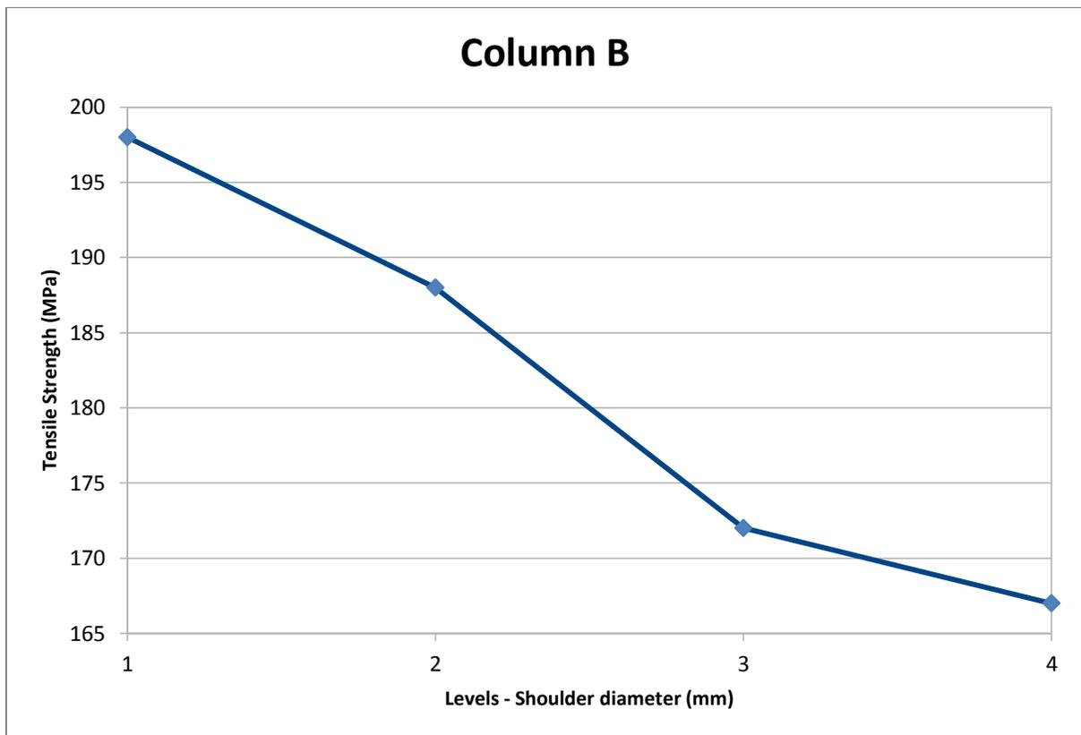
Fig. 1(c): Tensile strength as a function of tool shoulder diameter
