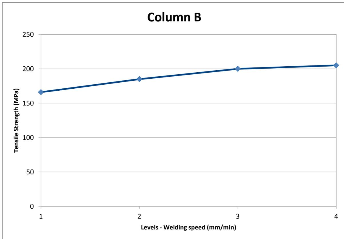
Fig. 1(a): Tensile strength as a function of welding speed
