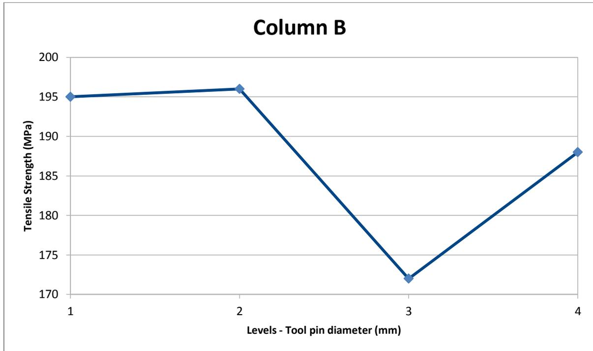
Fig. 1(d): Tensile strength as a function of tool pin diameter
