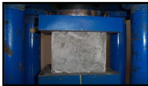
Figure: - 3. Testing Of Concrete Cubes
