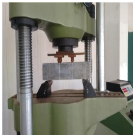
Figure 4: Prism Testing in UTM
