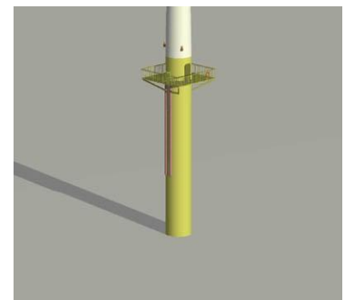
Figure 2: A typical Monopile Support Structure [19]
