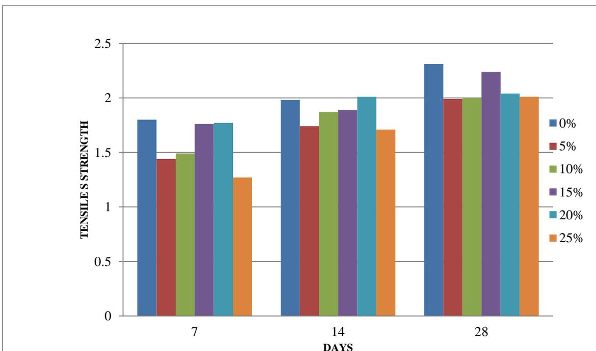
“Figure 5. Tensile Strength Of Cylinder For All Ratios Replacement Of Cement By Wa”.
