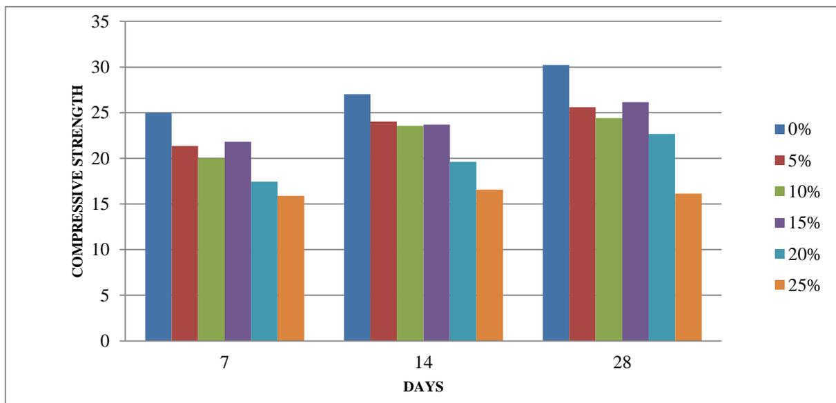
*Figure 4. Compressive Strength Of Cube For All Ratio Replacement Of Cement By WA*
