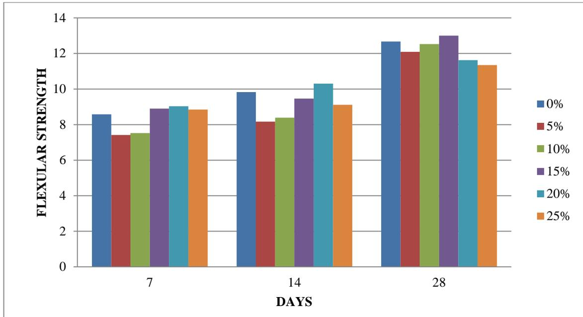
“Figure 5. Flexural Strength Of Beam For All Ratios Replacement Of Cement By WA”.
