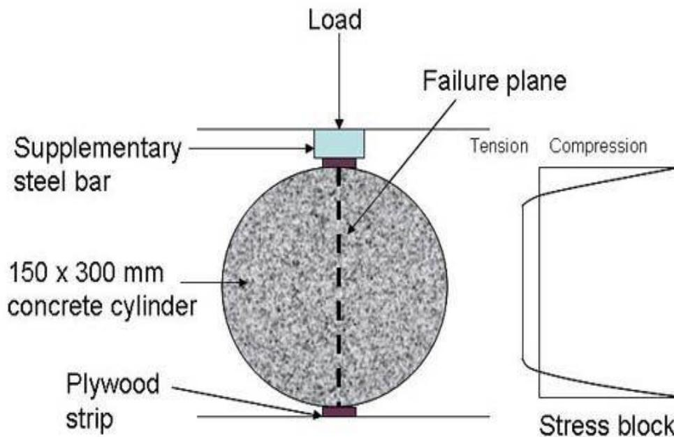
*“Figure 3. Load Application on Cylinder”.*
