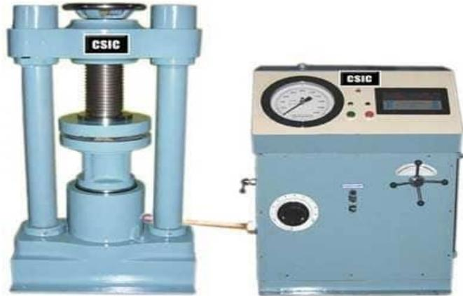
“Figure 1. Compression Testing Machine”.
