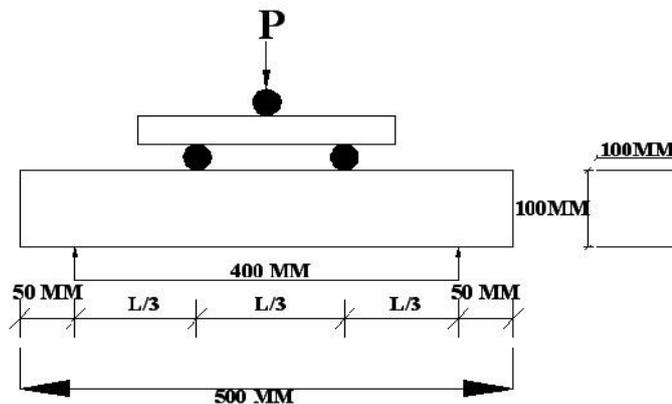
“Figure 2. Load Application on Beam”.
