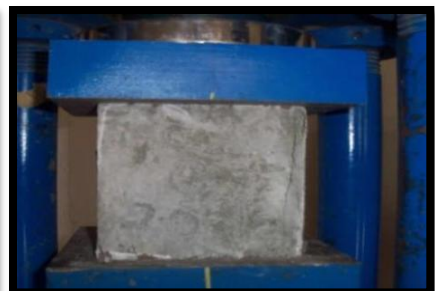
Figure: -6.Testing Of SCC Cubes
