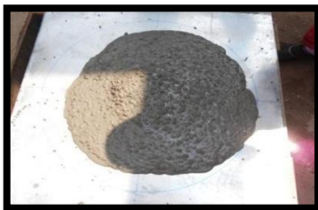
Figure: -1.Slump Flow test
