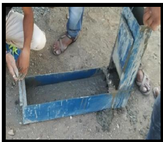
Figure: -4.L- Box Test
