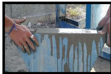
Figure: -2.V-Funnel Test
