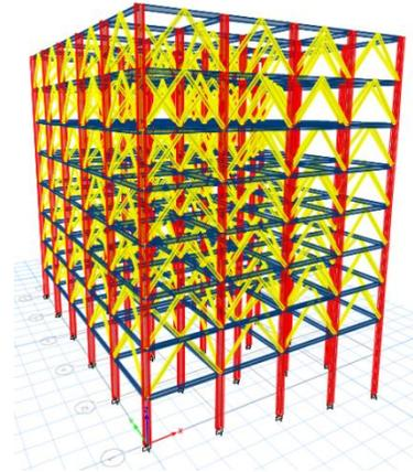
Frame-5 Chevron (Inverted V) braced frame
