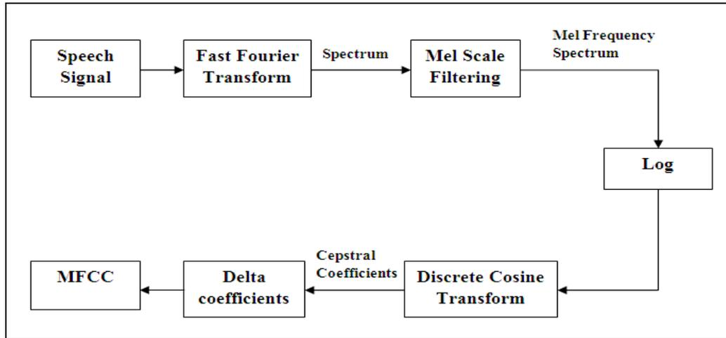
Figure2. Block diagram for extracting MFCC features
