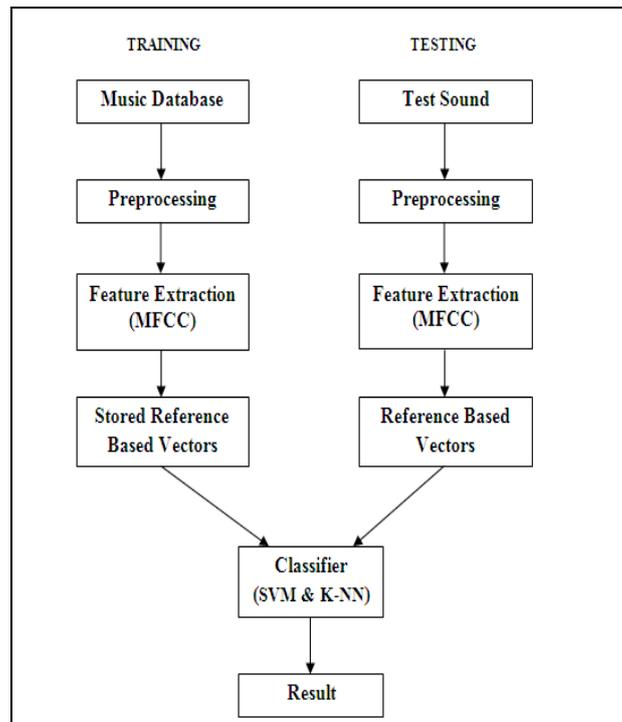
**Figure 1. General block diagram of proposed Musical Instrument Recognition system.**
