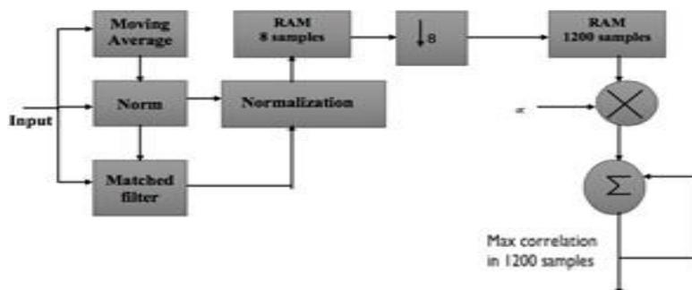
Figure 4. Area efficient PSS detection architecture
