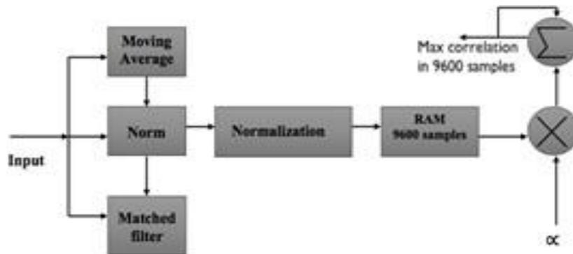
Figure 3. PSS detection architecture.
