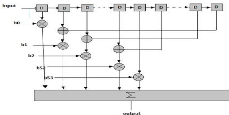
Figure 5. Centrally symmetric matched filter
