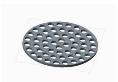
Fig.2 Fifty five Cavity Bakelite Fixture for Rubber bushes
